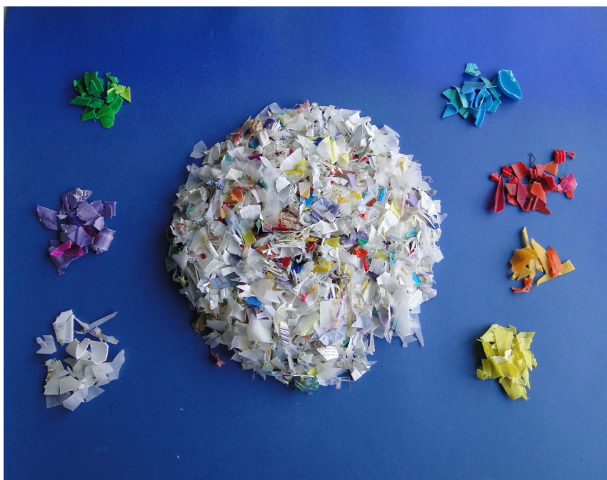
Fraunhofer LBF has developed technologies and processes for determining recycle content. Shown are samples before analysis. Courtesy of Fraunhofer LBF
