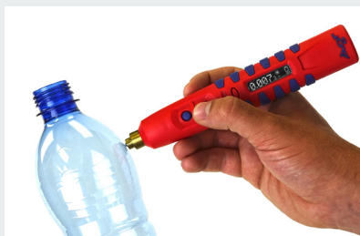
Agr's ThicknessPen is lightweight, portable and can be used in capacitive or magnetic measurement modes. Courtesy of Agr International
