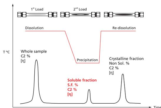
Elution of the whole sample and PP fractions in a TREF column
